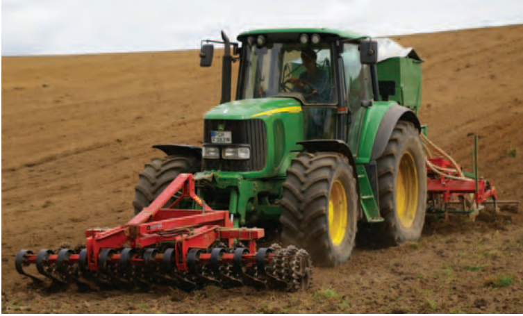
Figure 17.15 Seedbed preparation. Several stages of the process are completed in a single pass
