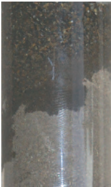
Figure 19.2 Wetting front. As water is added to a dry soil it soaks into the soil with a clear line that can be seen between the unchanged (dry) soil and the saturated soil above
