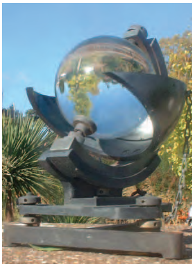
Figure 2.15 Campbell-Stokes Sunshine Recorder
