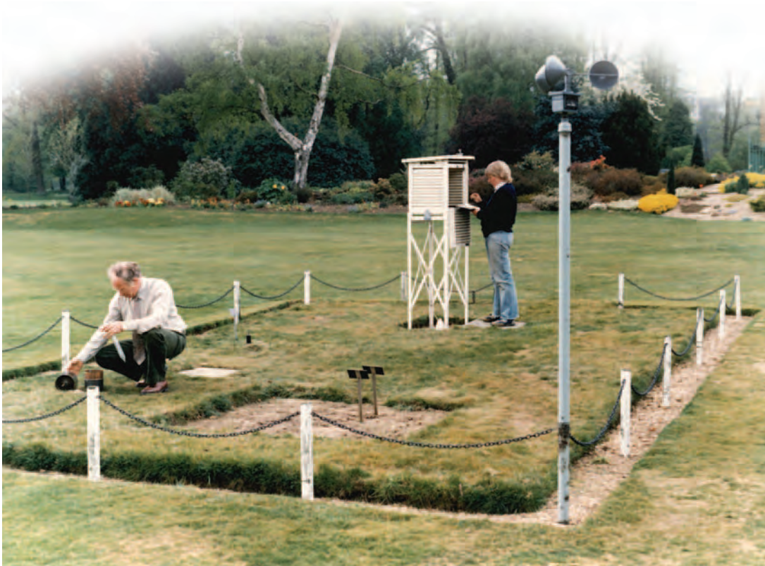
Figure 2.1 Agrometeorological station showing rain gauge (left), Stevenson's screen (centre) and anemometer (right).
