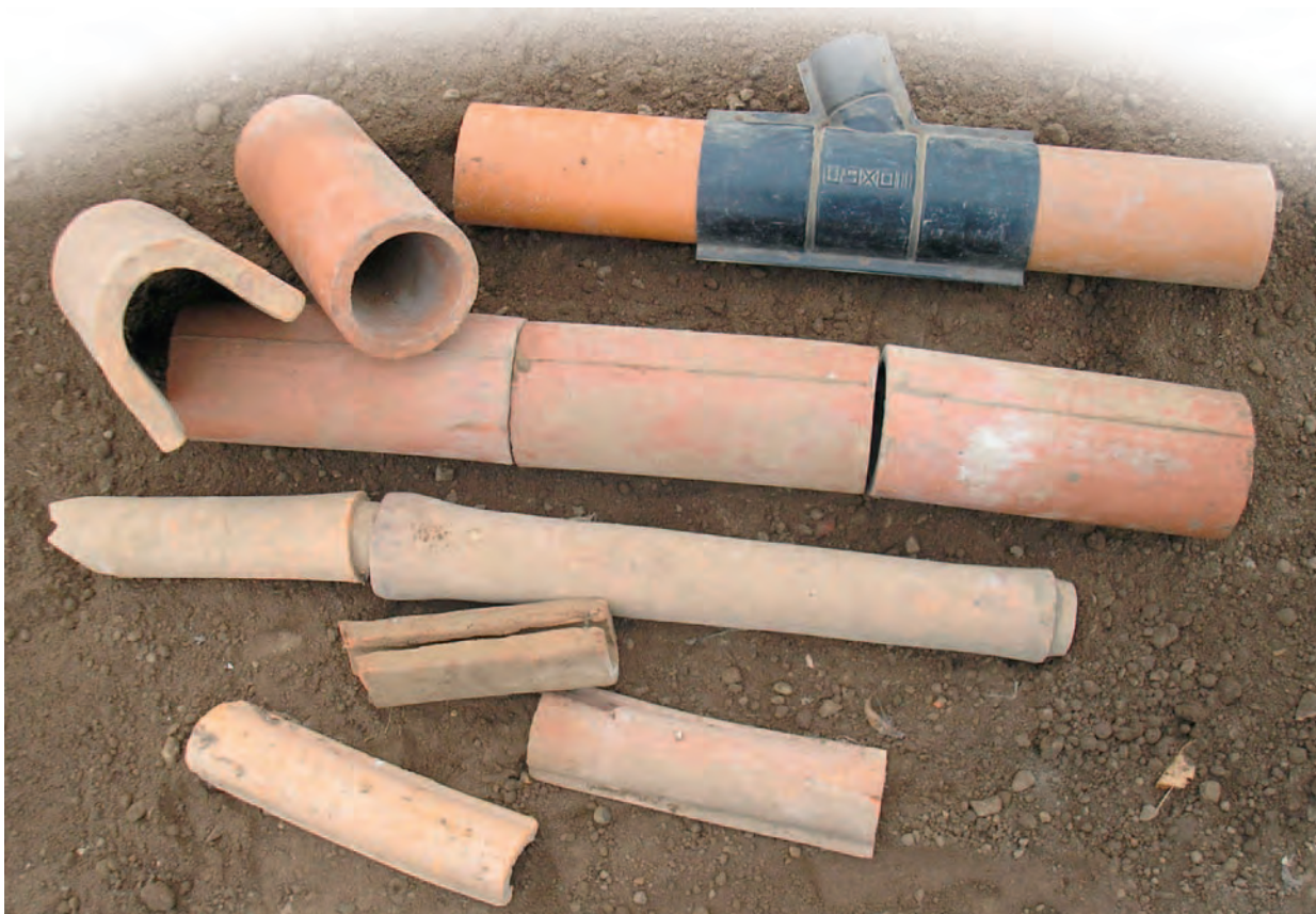
Figure 19.1 Drainage pipes. Modern clay pipes shown in the centre are butted up close together. An older method is shown below it and modern plastic piping is shown above. In the top left is a view of the modern clay pipe alongside the old 'horse shoe' tile (it would have sat on a 'mug plate' to prevent moving water washing away soil) and at the bottom are smaller examples of this type of old pipe
