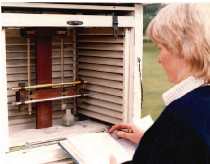
Figure 2.12 Stevenson's Screen showing Max-Min Thermometer (horizontal) and Wet and Dry Thermometer (vertical).
